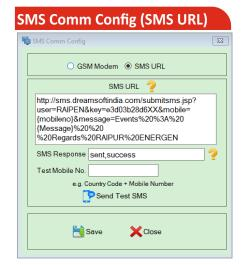
If Web Based API is used to relay Alarm SMS then that URL Settings can be done here. User will require Internet for this Option to relay SMS.
