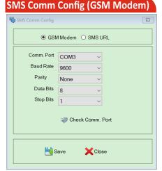
If Modem is used to relay Alarm SMS then Modem Settings can be done here. Modem with a SIM Card is the preferred option to relay Alarm SMSes.
