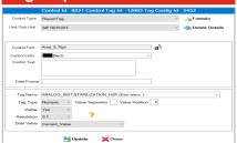
Tag Settings which user can map with respect to Unit / Sub Unit. Data Value can be selected which needs to be displayed i.e Current Value, First Value etc.
