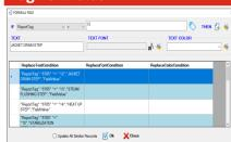
User can write Formulas to Compare Tag Value with Pre Defined Value and Change Text, Fonts, Colour etc, Convert Digital Tag into String, Multiple Comparisions etc.
